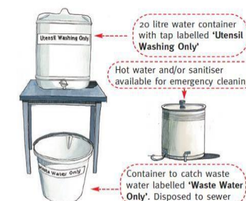
Two containers of sufficient capacity are to also be provided for adequate cleaning of utensils Figure 2 – Minimum utensil washing facilities
